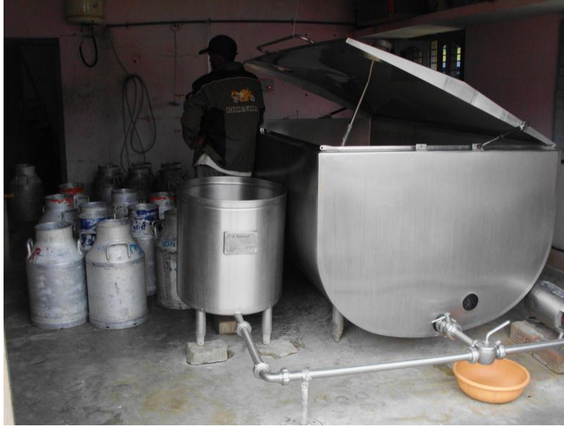
FIGURE 1. Bulk Milk Chiller
